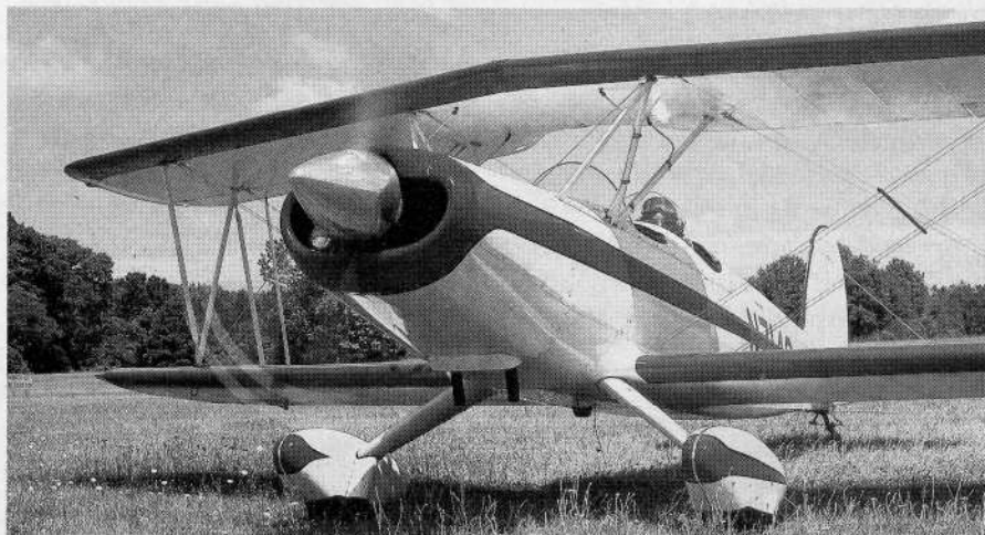
The engine swings a 72-inch Hartzell propeller.
