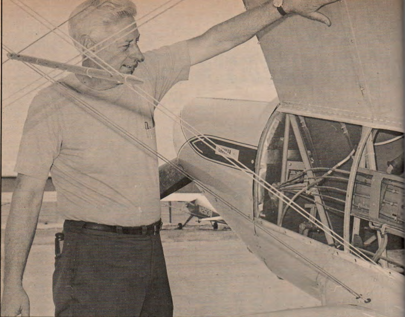
Designer-owner Ed Marquart shows how the side panels can be lifted on the Charger for easy maintenance.
