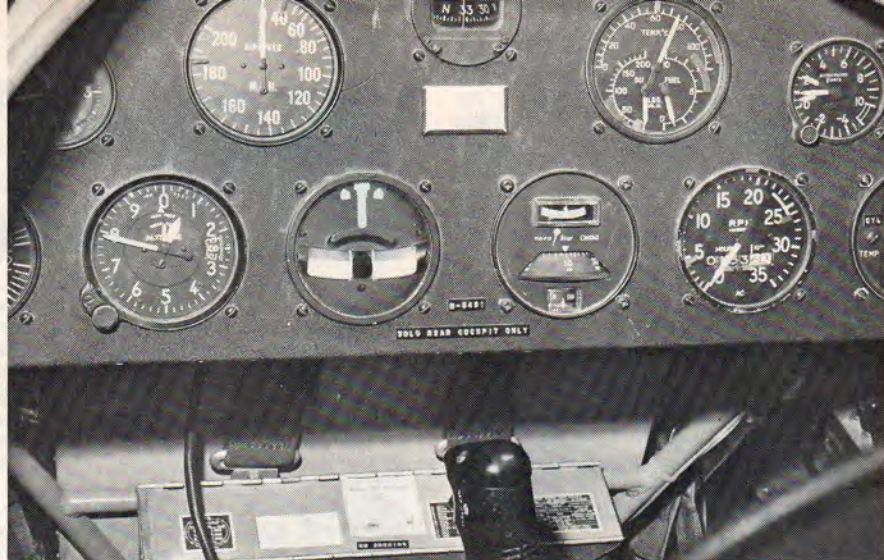
Just below this rear panel of the Charger is a small radio. The "G" meter isn't redlined but the little homebuilt is rated for maneuvers ranging from +6 to -4½ Gs.
