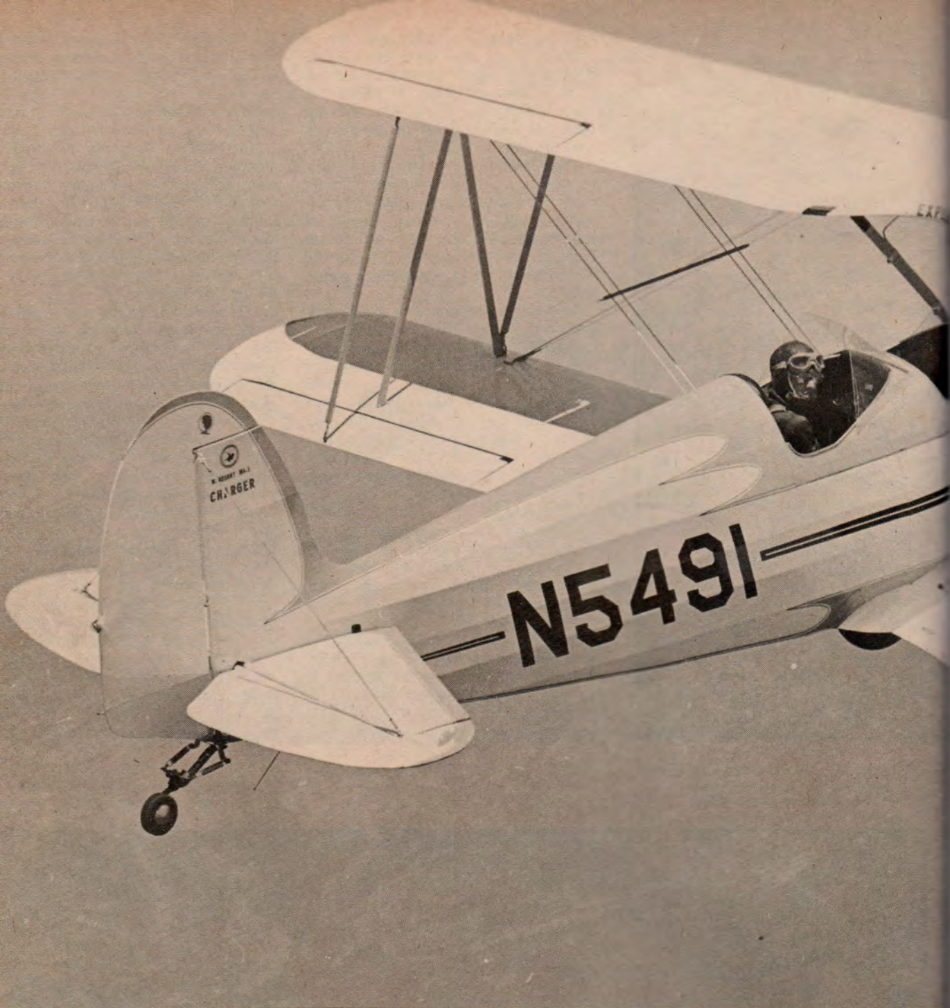
Solo is from the rear seat only but the four-cylinder 125-hp Lycoming has plenty of umph to carry two big people at a cruising speed of 115 mph on a hot day.
