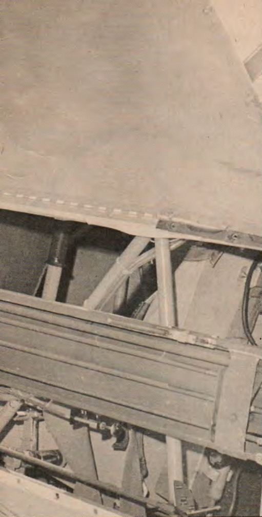
Oil on the fuselage is prevented by exhausting the breather tube by a wheel.
