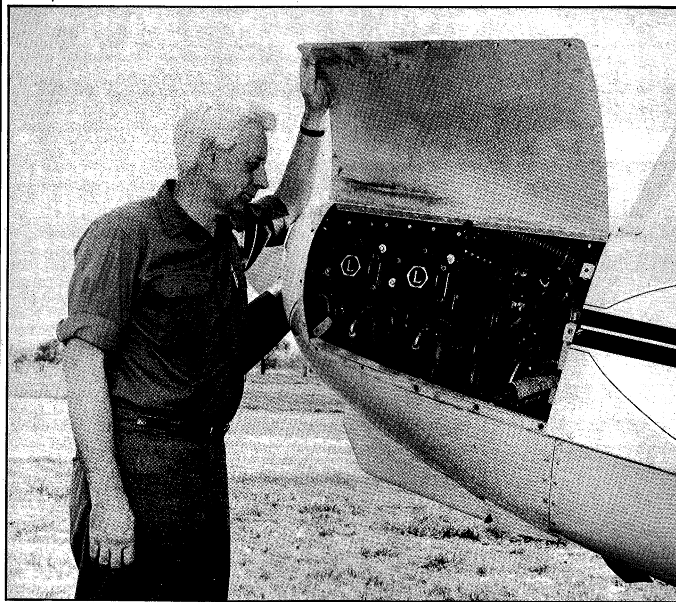
125-hp Lycoming O-290-1 swings a metal McCauley prop, a combination that gives smooth performance in cruise or aerobatics.
